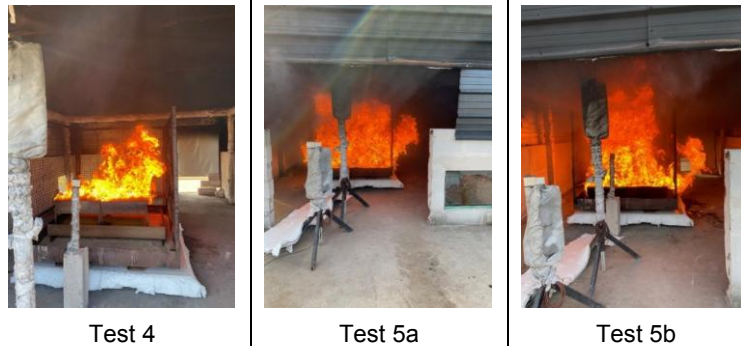
Figure 3: Flames observations of pool fire with tray surface above 0.9\text{m}^2
